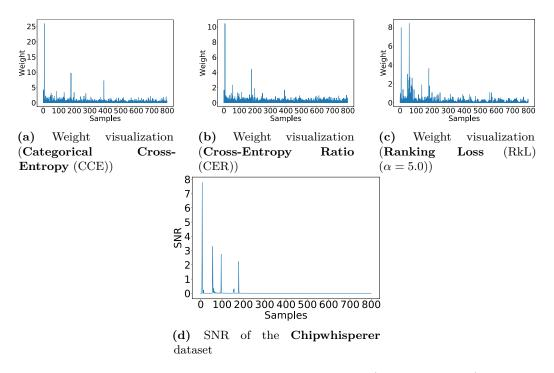
Figure 1: Visualization of the approximation error (Chipwhisperer)
