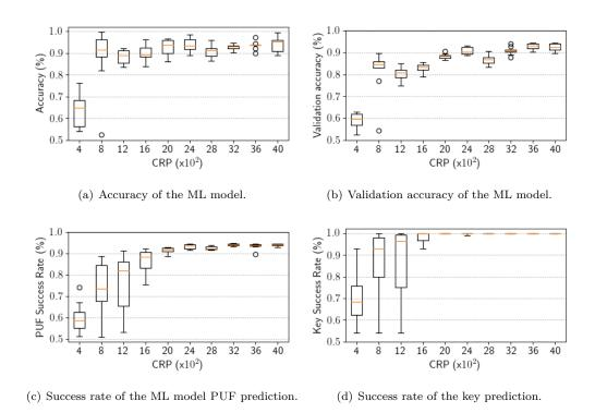
**Figure 4:** Evaluation of the attack idea using a repetition code with n = 7, Arbiter PUF model with 128 bit challenge, and a Siamese neural network. For every number of CRPs ten neural network were trained and evaluated.
