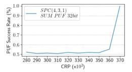
**Figure 7:** PUF success rate of two attacks on a 32-SUM PUF while utilizing XOR-equations with  $\kappa = 3$  of the SPC(3, 2, 1) and  $\kappa = 4$  of the SPC(4, 3, 1) code.
