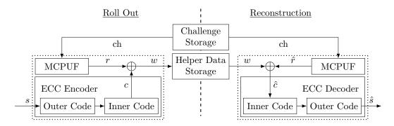
**Figure 1:** Visualization of the key-storage scenarios with PUFs: At some point in time – during *Roll Out* – a key is stipulated for the device. Later – during *Reconstruction* – the key is derived from the noisy PUF, given public helper data and challenges.
