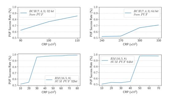
**Figure 8:** PUF success rate of attacks on a 32-SUM PUF and a 64-SUM PUF while utilizing XOR-equations with  $\kappa = 4$  of the RM(16, 4, 8) code and the BCH(7, 4, 3) code.
