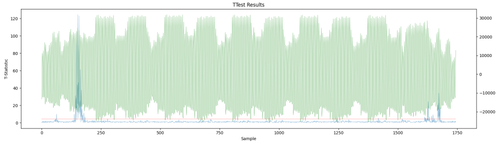
(b) Side-channel protected implementation TVLA results after 100K traces.
