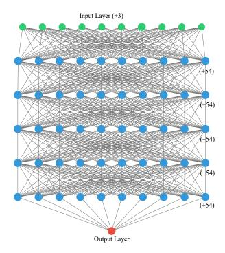
Fig. 1: Fully Connected Neural Network
