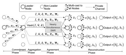
Figure 3: Messages sent during each phase of the SPURT. We describe contents of the messages i.e., the notations over the arrows in §V.
