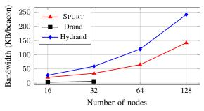
Figure 5: Average bandwidth usage (sent + received data) measured in Kilobytes per beacon output with varying number of nodes.
