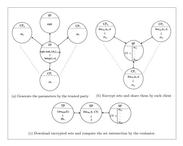
Fig. 3: The process of how to use our scheme
