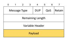
Fig. 4: The packet of MQTT
