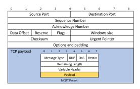
Fig. 5: An MQTT packet on a TCP network
