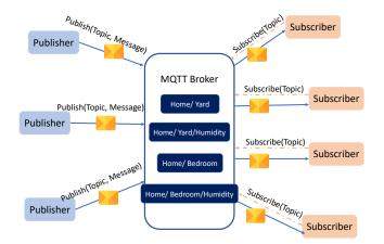
Fig. 6: The message transport in MQTT
