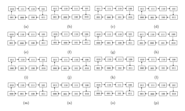
Figure 7: State diagrams of the 3-stage 1-terminal-bit Galois NFSR in Example 4
