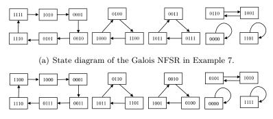
(b) State diagram of the Fibonacci NFSR in Example 7.
