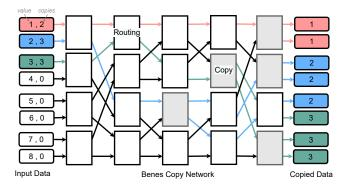
**Figure 5:** Benes copy network. Each intermediate node is a controlled swap gate that either routes the inputs or copies one of the inputs to output wires. Each input node has a value and number of copies. First element is copied twice while element two and three are each copied three times.
