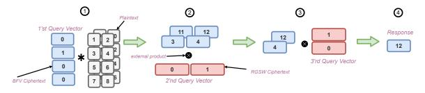
**Figure 3:** Examples of different variants of three dimensional hierarchical PIR. In the top figure the client queries are composed of all RGSW ciphertexts and the output of each dimension is BFV ciphertexts. In the bottom figure, first dimension's query vector consists of BFV ciphertexts, remaining query vectors are still RGSW ciphertexts and the first dimension is slightly larger than the other dimension.
