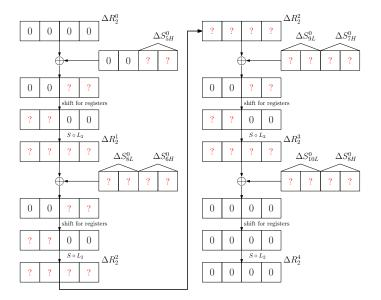
Figure 4: The difference transitions in FSM for the first 4 clocks.
