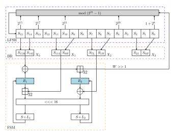
Figure 1: The initialization phase of ZUC-256.
