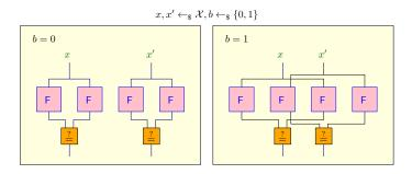
**Fig. 6.** In a given group of circuits, depending on the value of *b*, the leftmost and rightmost circuits (outer circuits) are paired with the circuits in the middle (inner circuits). Circuits in a pairing are given the same input, and their outputs are checked for equivalence.
