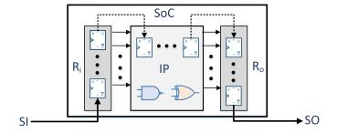
Fig. 1. Scan-based IP access for logic-locking attacks.
