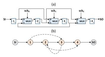
Fig. 6. (a) Sample scrambled scan-chain corresponding to Figure 5 and (b) Corresponding *scramble-digraph*
