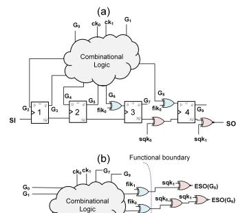
Fig. 3. (a) Proposed SeqL-style locking (b) Scan-unrolled equivalent
