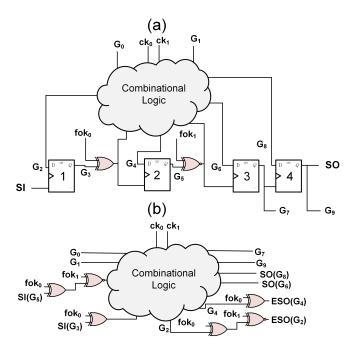
Fig. 2. (a) EFF-style locking (b) Scan-unrolled equivalent
