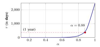
Fig. 13. Estimated decryption time  $(\tau = \tau_0 * 2^{\lfloor \frac{\alpha \cdot n + 1}{3} \rfloor})$  for b04 (the smallest circuit under consideration for scrambling), as a function of areacost constraint  $\alpha = \frac{\eta}{n}$  (0 <  $\alpha \le 1$ ). Please note the Y-axis range.
