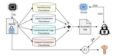
Fig. 8. Formulation of SAT-attack on Scan-Scrambling.
