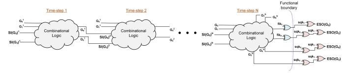
Fig. 12. Time-unrolled locked netlist used for multi-cycle-attack. Primary inputs are same for all time-frames, because input-register  $R_i$  (shown earlier in Figure 1) is scanned-in only once before first capture cycle. Primary outputs of intermediate stages are not observable because output-register  $R_o$  is scanned-out only once after the last  $(N^{th})$  capture cycle.
