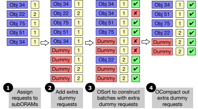
Figure 5. Generating batches of requests at the load balancer.
