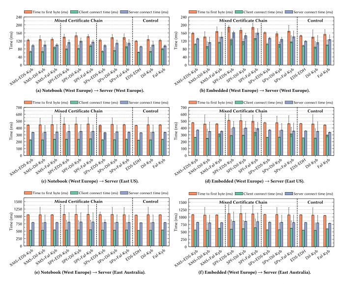
Figure 3: Time measurements under realistic network conditions at increasing client-server distances (median times in ms; error bars for 25th and 75th percentile).
