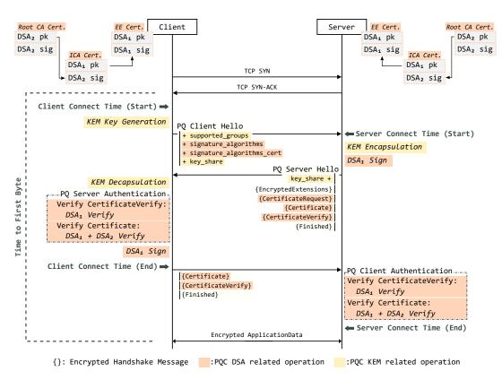
Figure 1: Post-quantum TLS 1.3 handshake illustrating the concept of mixed certificate chains.
