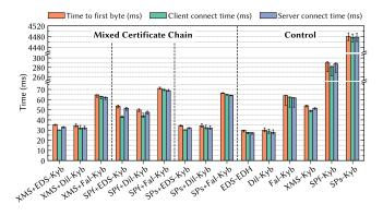
Figure 2: Time measurements in the local setting (median times in ms; error bars for 25th and 75th percentile): Embedded  $\rightarrow$  Notebook.
