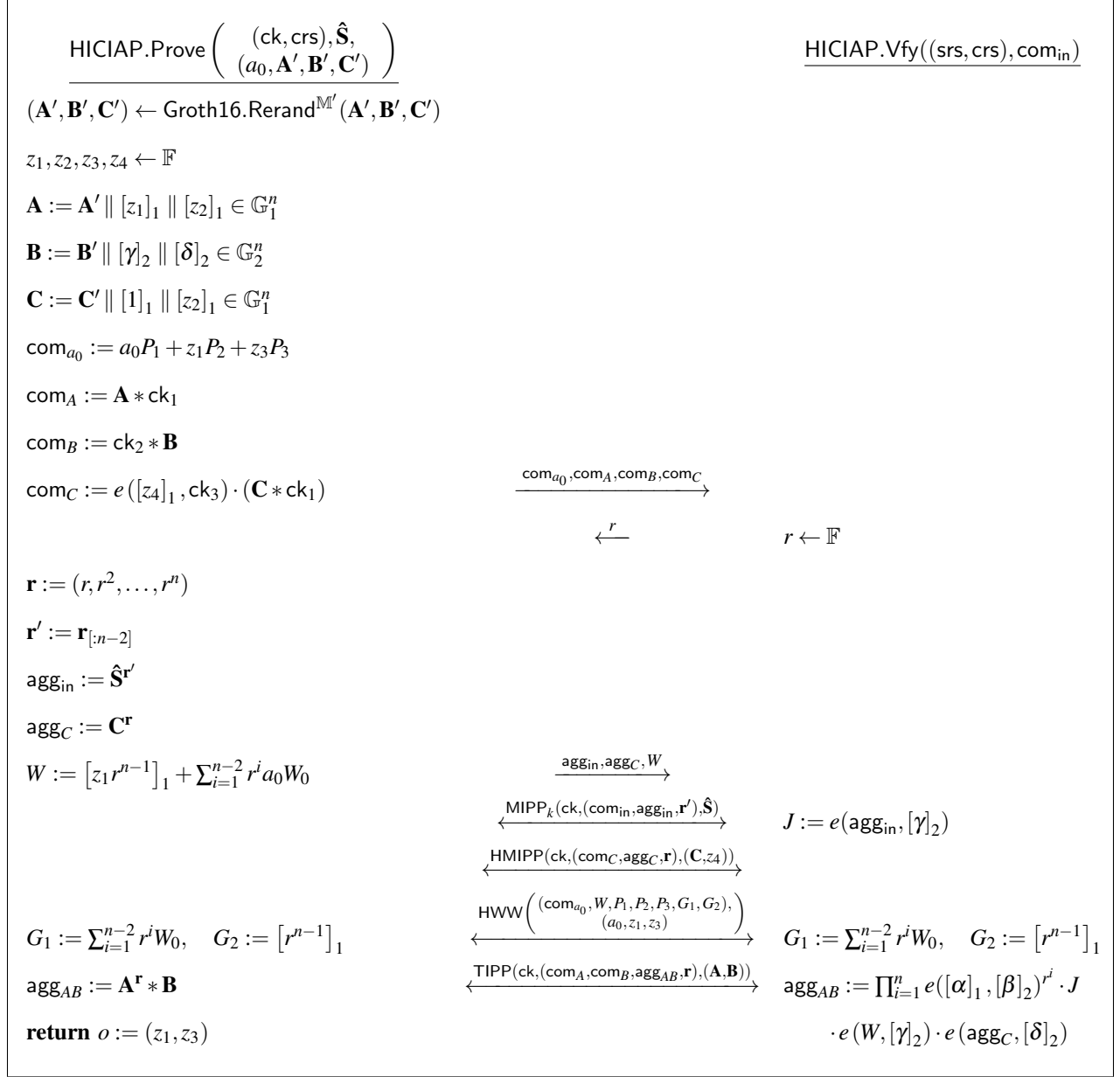
Fig. 4: The (interactive) HICIAP protocol. Vfy accepts iff all subprotocols MIPP, HMIPP, HWW, and TIPP accept. The group elements W_0, [\alpha]_1, [\beta]_2, [\delta]_2, [\gamma]_2 are supplied by crs. The values P_1, P_2, P_3 used to compute \text{com}_{a_0} is a Pedersen commitment basis. The Rerand procedure is only executed on the indices in the (log-sized) masking set \mathbb{M}' = \mathbb{M} \cup \{n-2\} , where \mathbb{M} is defined in the proof of Lemma 4. It is the identity function everywhere else.
