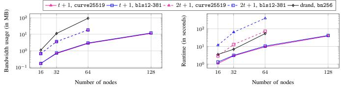
Figure 4: Bandwidth usage, amount of data sent by a node during ADKG protocol.
