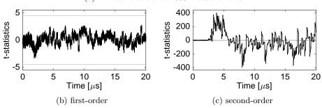
Fig. 6: Experimental analysis of our first-order PRESENT nibble-serial encryption design (covering the first five rounds); fixed vs. random t-test results using 100 million traces.
