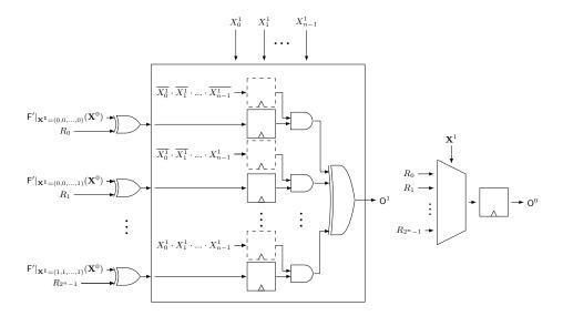
Fig. 4: General GHPC<sub>LL</sub> design with reduced latency.
