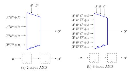
Fig. 3: Examples for first-order PINI-secure GHPC constructions.
