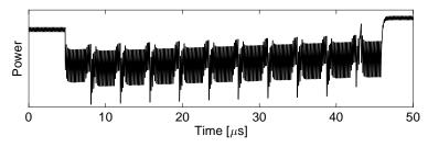
(a) A mean trace over 1000 measurements indicating the cipher rounds
