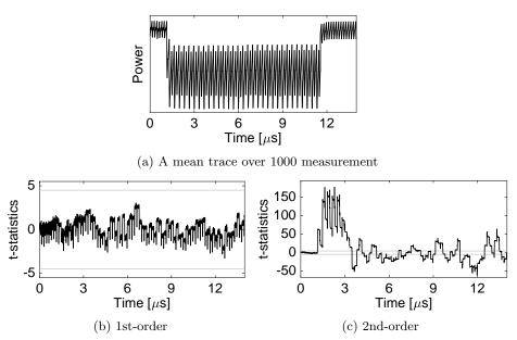
Fig. 7: Experimental analysis of our first-order PRESENT round-based encryption design (covering the entire encryption); fixed vs. random t-test results using 100 million traces.
