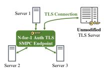
Fig. 1: TLS-in-SMPC's system architecture.
