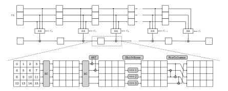
Fig. 2: The hight-level structure of SKINNY-n-3n and its round function (Thanks to https://www.iacr.org/authors/tikz/).
