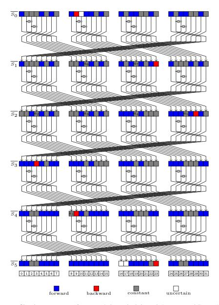
Fig. 24: Chunk separations of  $\tt AES-256$  's key schedule with Leurent and Pernot's representations
