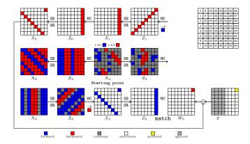
Fig. 20: The Meet-in-the-Middle attack on 6-round output transformation of Grøstl-256
