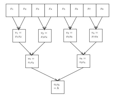
Fig. 1. An example of creation of auxiliary variables for m = 8.
