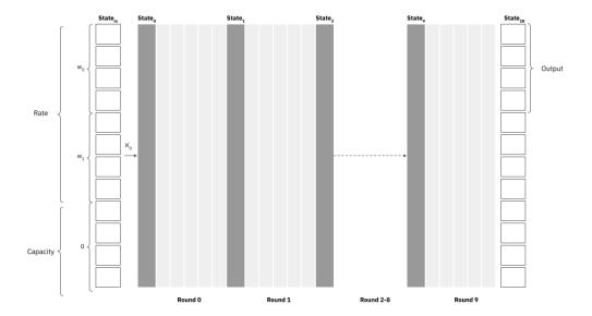
Figure 2: Instantiating the Rescue hash function as a sponge construction based on the Rescue permutation.
