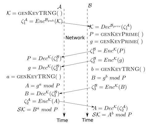
Fig. 1. Encryption-decryption using asymmetric and symmetric key to enhance Diffie-Hellman algorithm.
