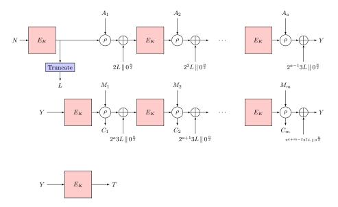
Fig. 1. The COFB mode of operation.
