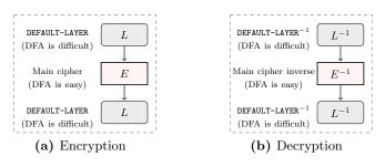
Fig. 1: Main cipher augmented by DEFAULT-LAYER to resist DFA
