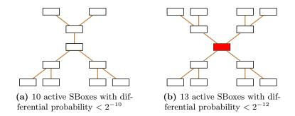
**Fig. 2:** 5-round differential characteristics (solid lines are active bits, white boxes are active SBoxes and red box is SBox with differential probability 1)
