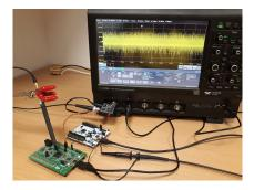
Figure 4: Experimental setup used for EM trace acquisition.
