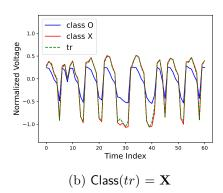
**Figure 9:** Matching the reduced template tr of a given attack trace with the reduced template of the two classes  $\mathbf{O}$  and  $\mathbf{X}$ .
