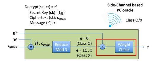
Figure 2: Pictorial Illustration of our PC oracle-based SCA on NTRU Prime
