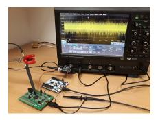
**Figure 4:** Experimental setup used for EM trace acquisition.
