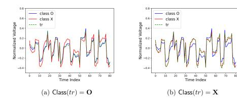
Figure 12: Matching the reduced template tr of a given attack trace with the reduced template of the two classes  $\mathbf{O}$  and  $\mathbf{X}$ .
