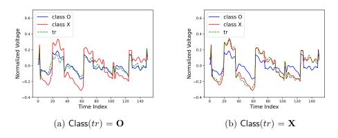
**Figure 6:** Matching the reduced template tr of a given attack trace with the reduced template of the two classes  $\mathbf{O}$  and  $\mathbf{X}$ .
