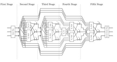
Figure 6: Representation of the S-box of design II. Register stages are denoted by dashed vertical lines.
