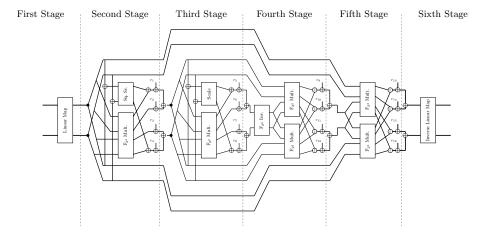
Figure 5: Representation of the S-box of design I. Register stages are denoted by dashed vertical lines.
