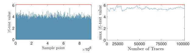
**Fig. 5.** A first-order leakage detection test based on 100,000 traces on the Picnic3. The |t|-value remains below 6.1 (as suggested by  $[DZD^+18]$ ), indicating the absence of exploitable first-order leakage for the 100,000 traces. Also, the maximum |t|-value is bounded and becomes stable with the increased number of traces (right).
