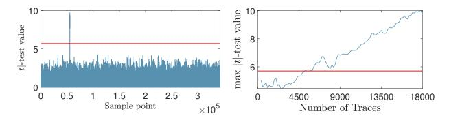
Fig. 2. A first-order RvR test on the unprotected Picnic3 implementation using revealed values from the online phase. The traces are classified based on a single bit of  $\hat{sk}K_0$ . Values above the 5.7 threshold (red line) indicate there are strong leakages (left). Also, the maximum |t|-value increases with respect to number of traces and the leakage becomes absolute after 6,000 traces (right).
