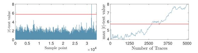
Fig. 1. A first-order RvR test on the unprotected Picnic3 implementation using revealed values from the offline phase. The traces are classified based on the bit  $\lambda_1^w + \cdots + \lambda_{16}^w$ . Values above the 5.7 threshold (red line) indicate strong leakage (left). Moreover, the maximum |t|-value increases with respect to the number of traces and the leakage becomes clear after 2,725 traces (right).
