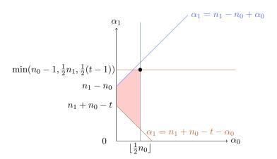
Figure 4: The feasible region defined by simplified constraint system. In this diagram, each of the constraints in Parameter Constrains D.2 is depicted with a corresponding line. For instance, Constraint 4 is depicted with the red decreasing line, and the feasible region must be above it.
