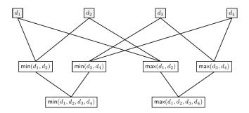
Fig. 2. Optimized  $\pi_{\min \max}$ : An example circuit to compute  $\pi_{\min \max}$  on an input vector of size n=4
