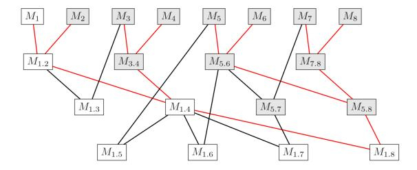
Fig. 3. ComposeNet $_{\lambda}$  for  $\lambda = 9$ . Computes the set of all matrix compositions  $M_1, M_{1.2}, M_{1.3}, \dots, M_{1.(\lambda-1)}$  [4]. The subgraph denoted in red computes ComposeNet<sub>\alpha</sub> for  $\alpha = 9$ ; the matrix composition  $M_{1,(\alpha-1)}$ .
