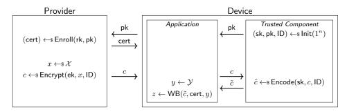
**Fig. 2:** Strong Global White-box (sGW) Scheme. For initial setup the provider runs the compiler program to generate the whitebox and some key material,  $(ek, rk, WB) \leftarrow sComp(F)$ . WB is distributed to all devices via a central appstore.
