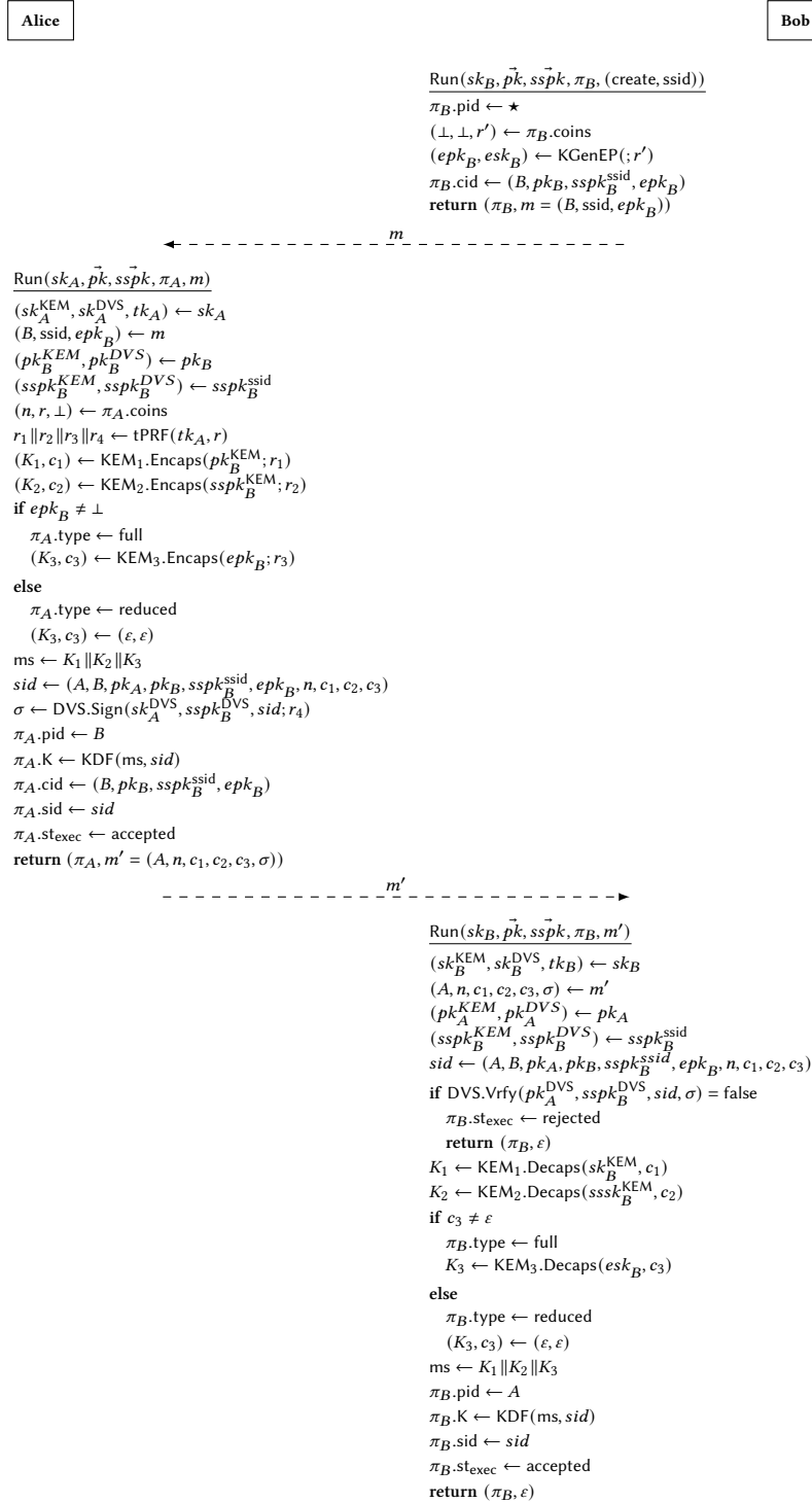
Figure 13: Formal specification of the Run algorithm of asynchronous DAKE SPQR wrt. the model given in Section 7. Note that the generation of long-term and semi-static keys during registration happens at the outset of the game \mathcal{G}_{\text{KE}}^{\text{ke-kind}}(\mathcal{A}) and the Signal Server is abstracted away. Thus these elements are not included explicitly in the above description.
