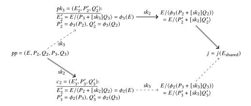
Fig. 18: Diagram of the underlying KE scheme of SIKE.
