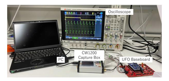
Fig. 10: Experimental setup overview.
