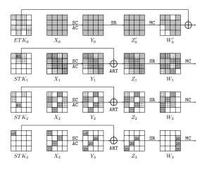
Fig. 14: Phase (1): The 4-round  $E_b$  of the attack on SKINNY-128-384.
