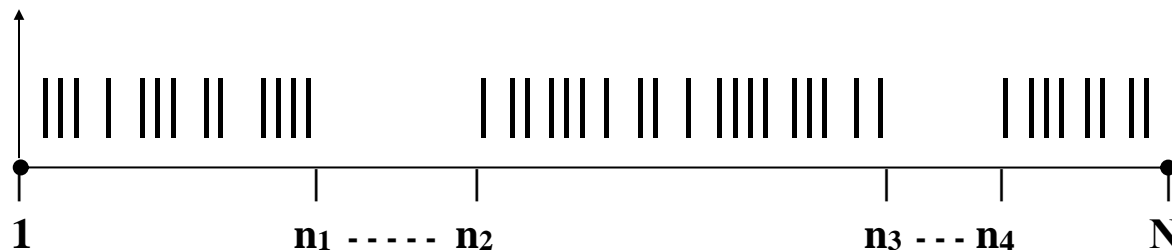
Figure 1. Random key sampling which leaves out two ranges of key values (from n_1 to n_2 and from n_3 to n_4 )
