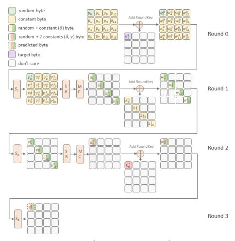
Fig. 2: Attacking  $k_0^0$  by targeting first byte  $(v_0^3)$  after  $S_3$ .
