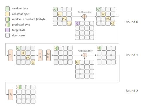
Fig. 1: Attacking  $k_0^0$  by targeting first byte  $(v_0^2)$  after  $S_2$ .
