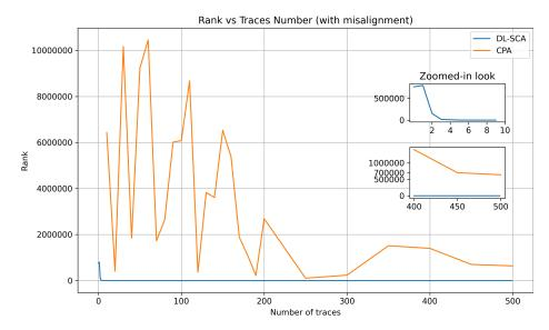
Fig. 6: DL-SCA and CPA on misaligned traces for key byte 0 after S-box on encryption round 3.
