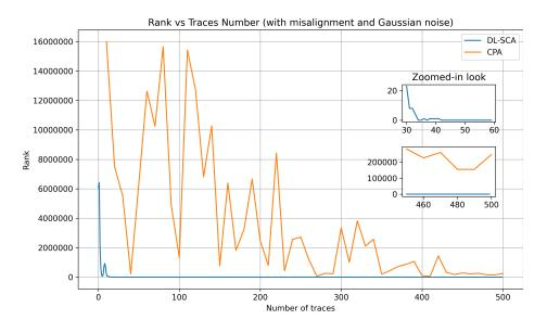
Fig. 7: DL-SCA and CPA on misaligned traces after adding Gaussian noise for key byte 0 after S-box on encryption round 3.
