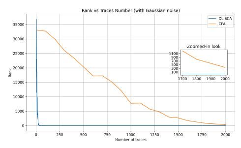
Fig. 4: DL-SCA and CPA after adding Gaussian Noise for key byte 0 after S-box on encryption round 2.
