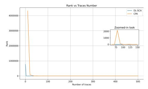
Fig. 5: DL-SCA and CPA on aligned traces for key byte 0 after S-box on encryption round 3.
