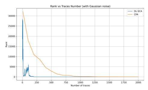
Fig. 3: DL-SCA and CPA for key byte 0 after S-box on encryption round 2.
