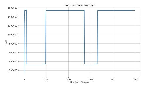
Fig. 8: DL-SCA on round 4 S-box with different plaintexts being used while training and constant plaintext used for attack. A fixed key was used both for profiling and for attack.
