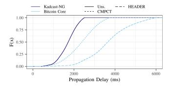
Figure 8: Block propagation delays for the QUIC-based kadcast-ng prototype and Bitcoin Core in a testbed of 1,000 nodes.
