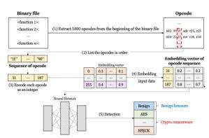
Figure 5 System diagram of transformer encoderbased crypto-ransomware detection for detection phase
