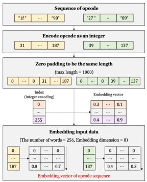
Figure 3 Opcode embedding process for input data pre-processing
