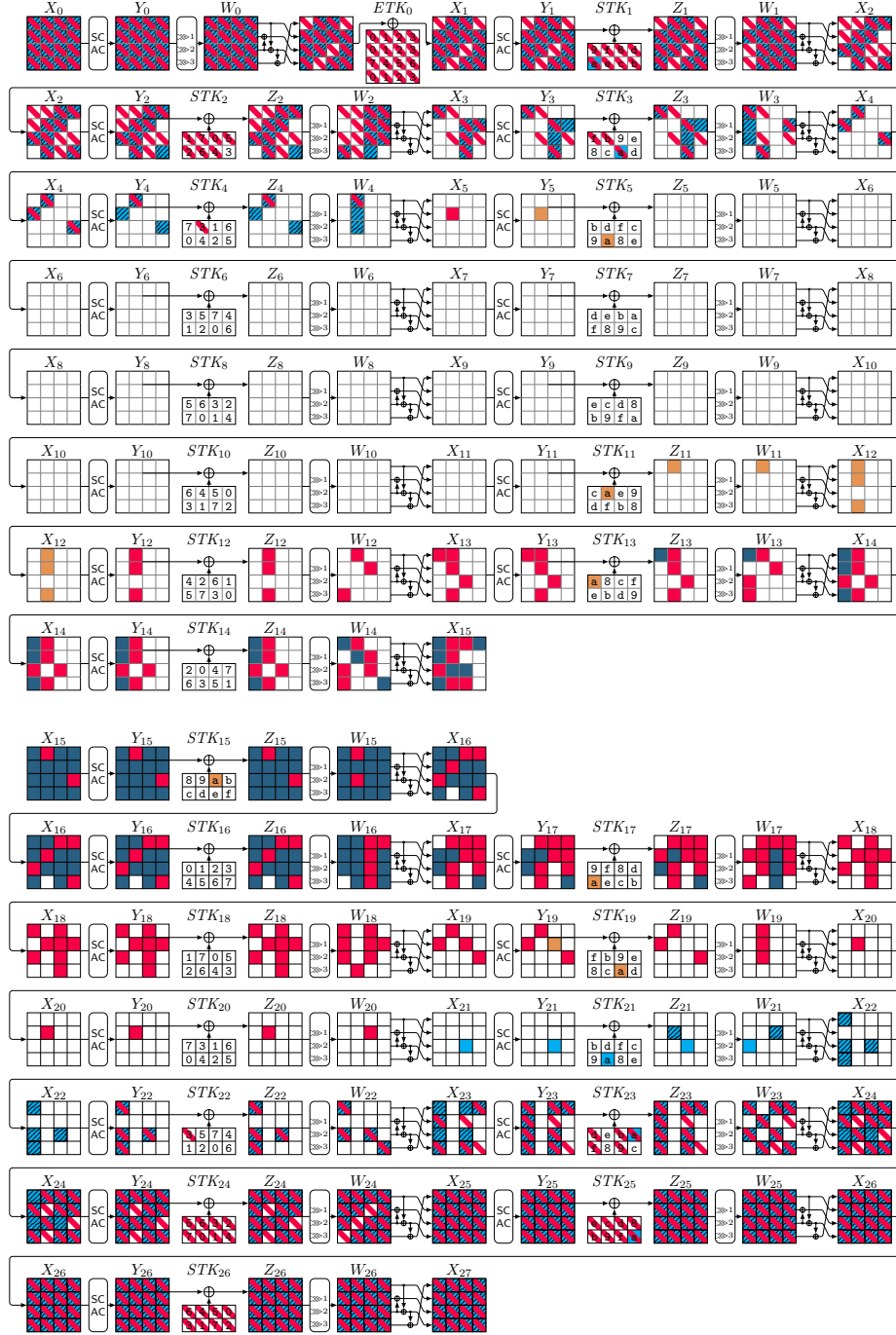
Fig. 9: ID attack on 27 rounds of SKINNY- n - 3n in the related-tweakey setting. |k_B \cup k_F| = 45 , c_B = 12 , c_F = 15 , \Delta_B = 12 , \Delta_F = 16 .
