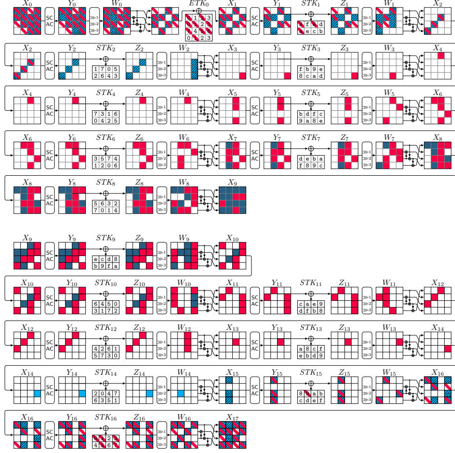
Fig. 6: ID attack on 17 rounds of SKINNY- n - n . |k_B \cup k_F| = 10 , c_B = 6 , c_F = 6 , \Delta_B = 7 , \Delta_F = 7 .
