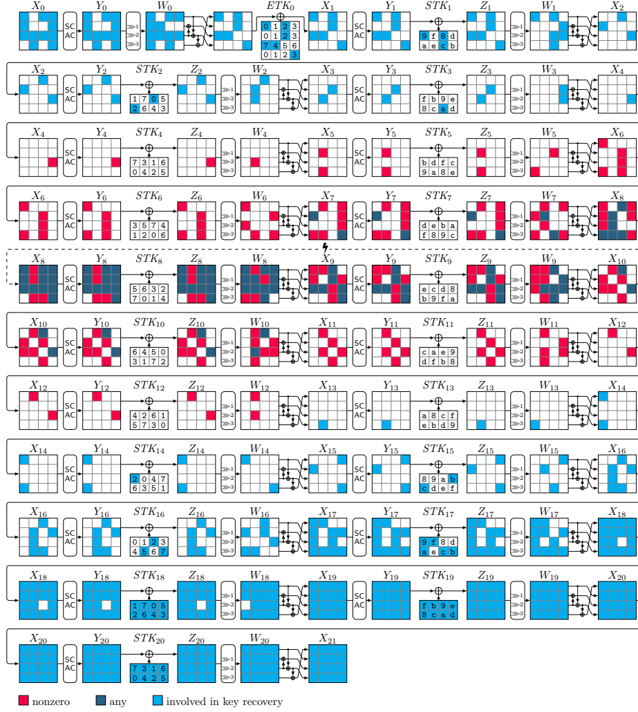
Fig. 13: ZC attack on 21 rounds of SKINNY- n - 3n . Number of actual involved key cells: 40
