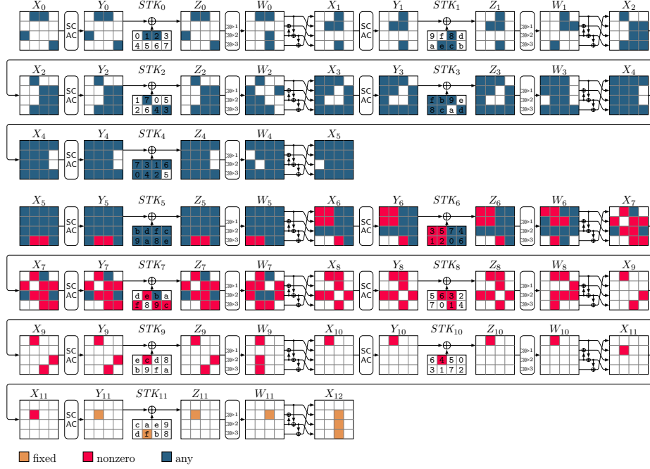
Fig. 16: ZC-Integral distinguisher for 12 rounds of SKINNY- n - n . STK[5] is active at most one time. X_{12}[6] \oplus X_{12}[10] \oplus X_{12}[14] is balanced. Data complexity: 2^{13 \cdot c} , c \in \{4, 8\} .
