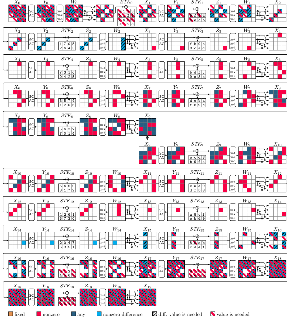
Fig. 8: ID attack on 19 rounds of SKINNY- n-2n , |k_B \cup k_F| = 26 , c_B = 6 , c_F = 15 , \Delta_B = 7 , \Delta_F = 16
