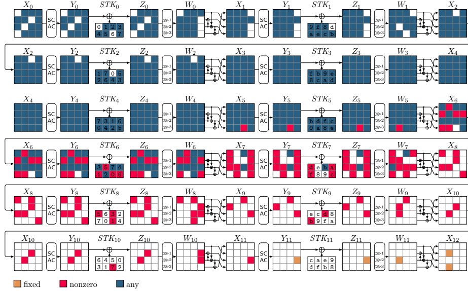
Fig. 17: ZC-Integral distinguisher for 12 rounds of SKINNY- n - 2n . STK[0] is active at most two times. X_{12}[5] \oplus X_{12}[13] is balanced. Data complexity: 2^{6 \cdot c} , c \in \{4, 8\} .
