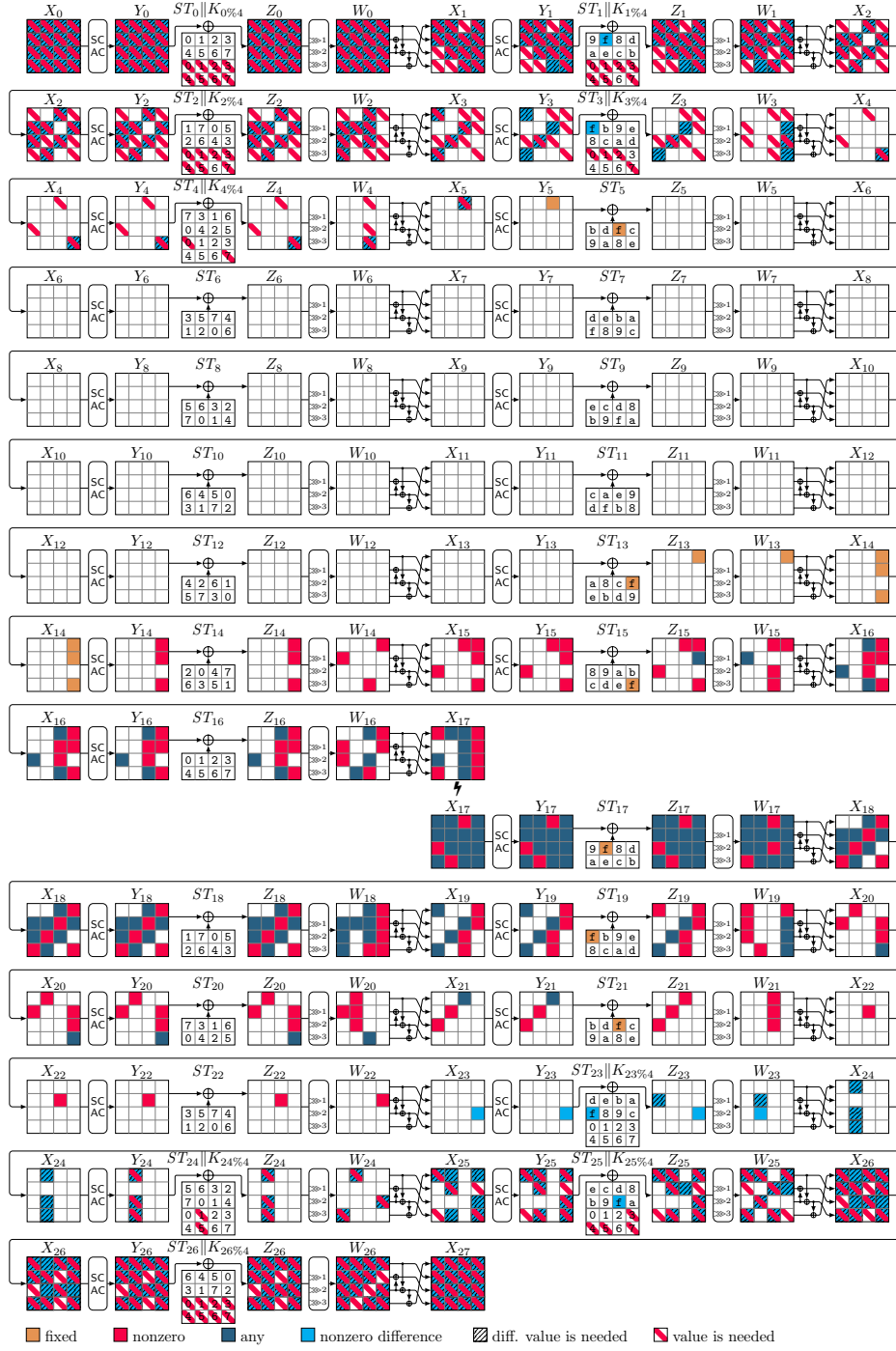
Fig. 41: ID attack on 27 rounds of SKINNY in the related-tweak setting. |k_B \cup k_F| = 27 , c_B = 12 , c_F = 12 , \Delta_B = 12 , \Delta_F = 13 .
