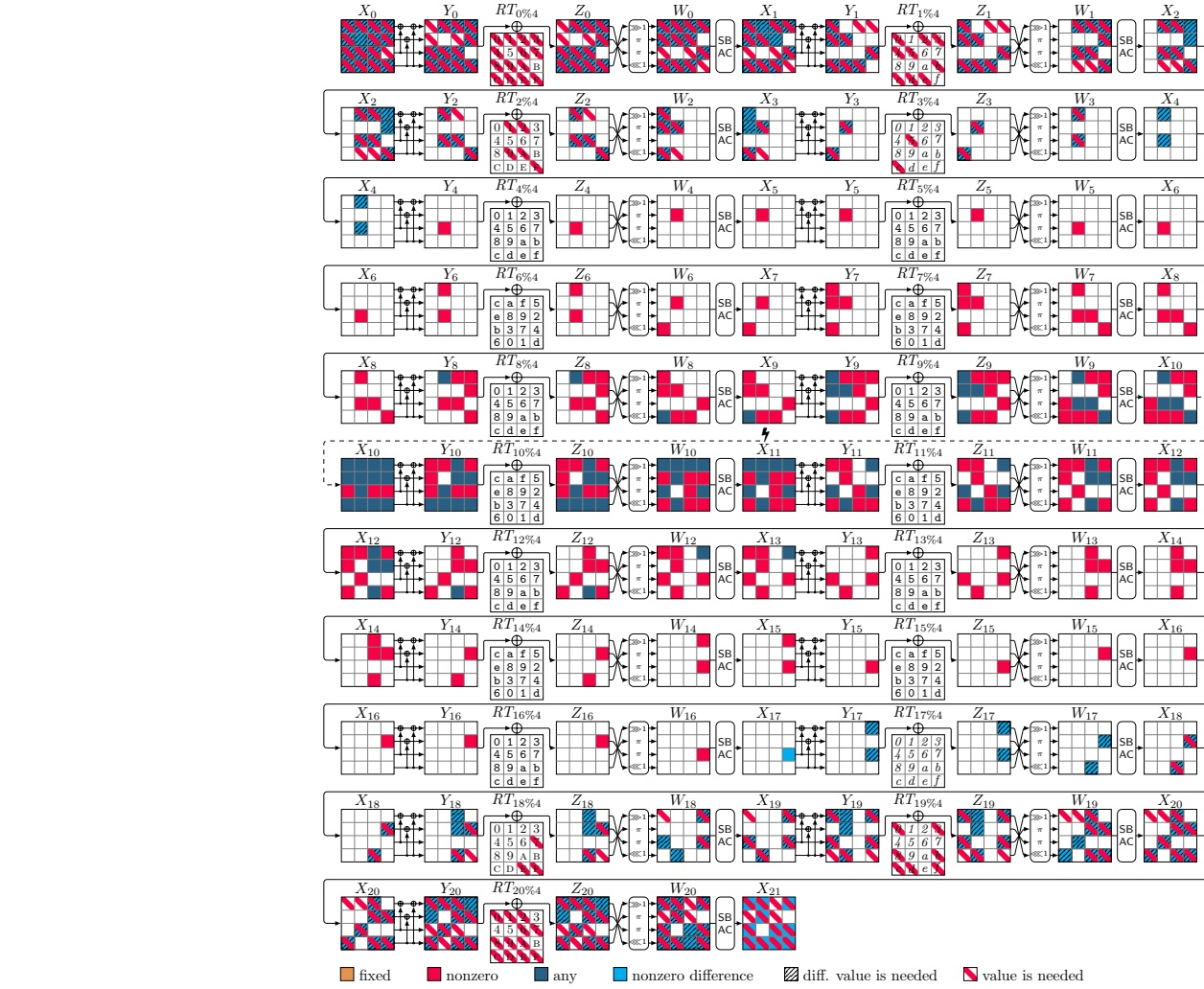
Fig. 31: ID attack on 21 rounds of CRAFT, |k_B \cup k_F| = 25 , c_B = 10 , c_F = 10 , \Delta_B = 11 , \Delta_F = 11
