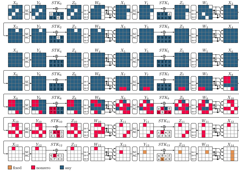
Fig. 20: ZC-Integral distinguisher for 14 rounds of SKINNY- n-3n . STK[0] is active at most three times. X_{14}[6] \oplus X_{14}[10] \oplus X_{14}[14] is balanced. Data complexity: 2^{7-c} .
