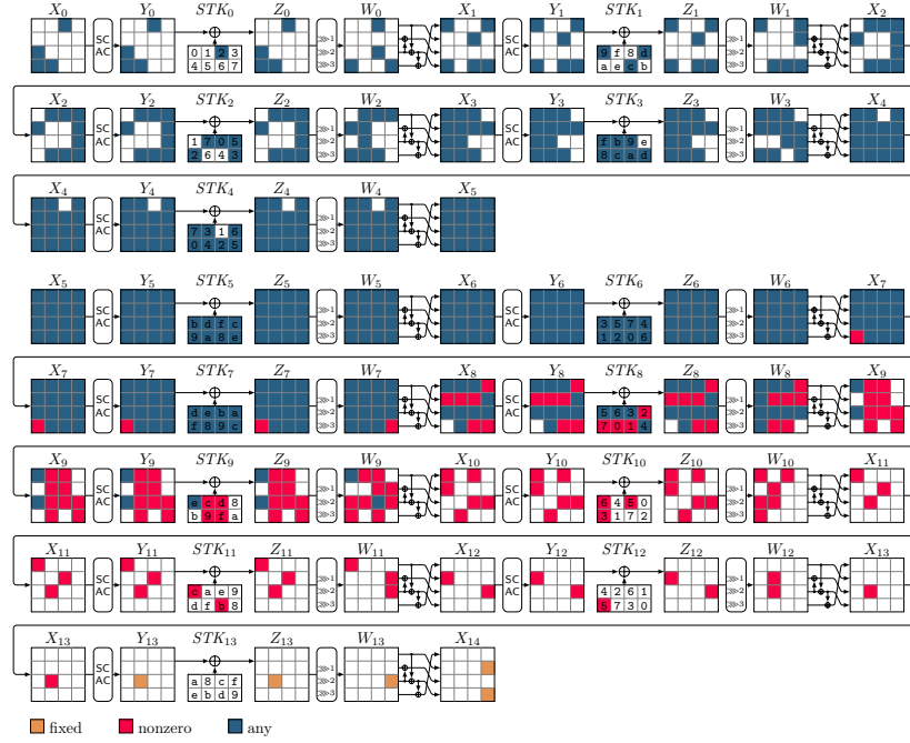
Fig. 19: ZC-Integral distinguisher for 14 rounds of SKINNY- n-2n . STK[1] is active at most two times. X_{14}[7] \oplus X_{14}[15] is balanced. Data complexity: 2^{14-c} , c \in \{4, 8\} .
