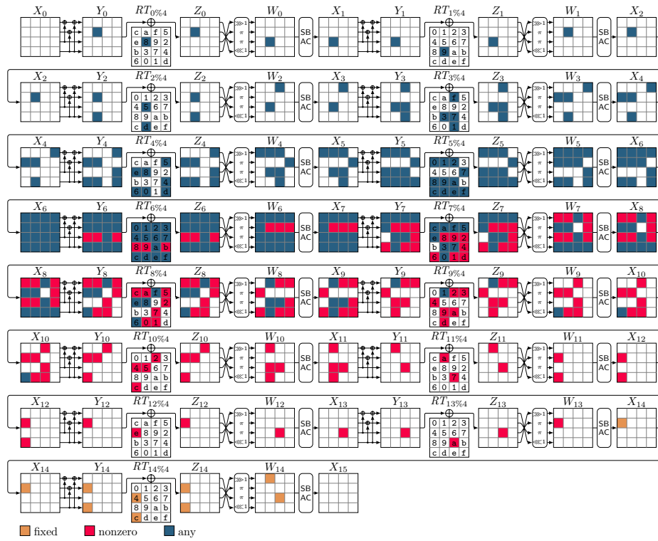
Fig. 35: ZC-Integral distinguisher for 15 rounds of CRAFT. \text{Offset} = 3 . RTK[b] is active at most one time. W_{14}[1] \oplus W_{14}[10] is balanced. Data complexity: 2^{64} .
