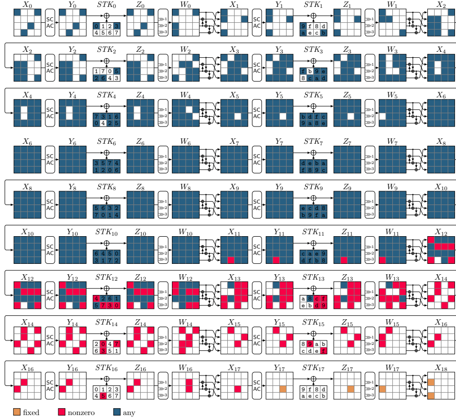
Fig. 31: ZC-Integral distinguisher for 18 rounds of SKINNYe/SKINNYe-v2. STK[4] is active at most four times. X_{18}[4] \oplus X_{18}[12] is balanced. Data complexity: 2^{64} .
