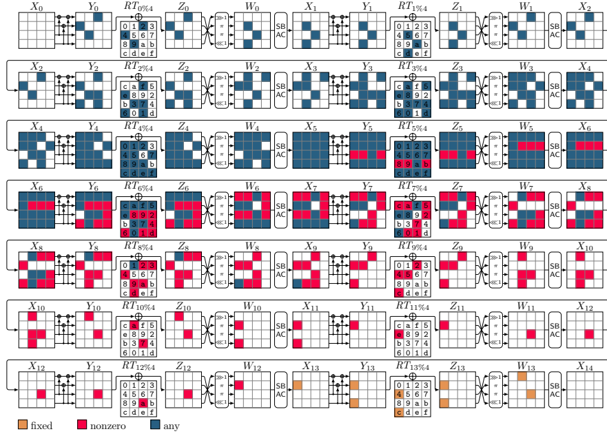
Fig. 37: ZC-Integral distinguisher for 14 rounds of CRAFT. \text{Offset} = 0 . RTK[b] is active at most one time. W_{13}[1] \oplus W_{13}[10] is balanced. Data complexity: 2^{56} .
