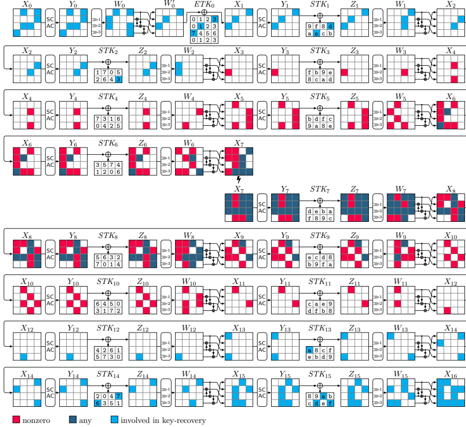
Fig. 11: ZC attack on 16 rounds of SKINNY- n - n . #Involved key cells: 8
