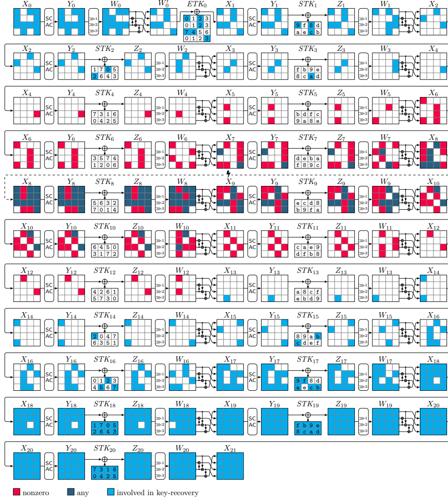
Fig. 13: ZC attack on 21 rounds of SKINNY- n-3n . #Involved key cells: 40
