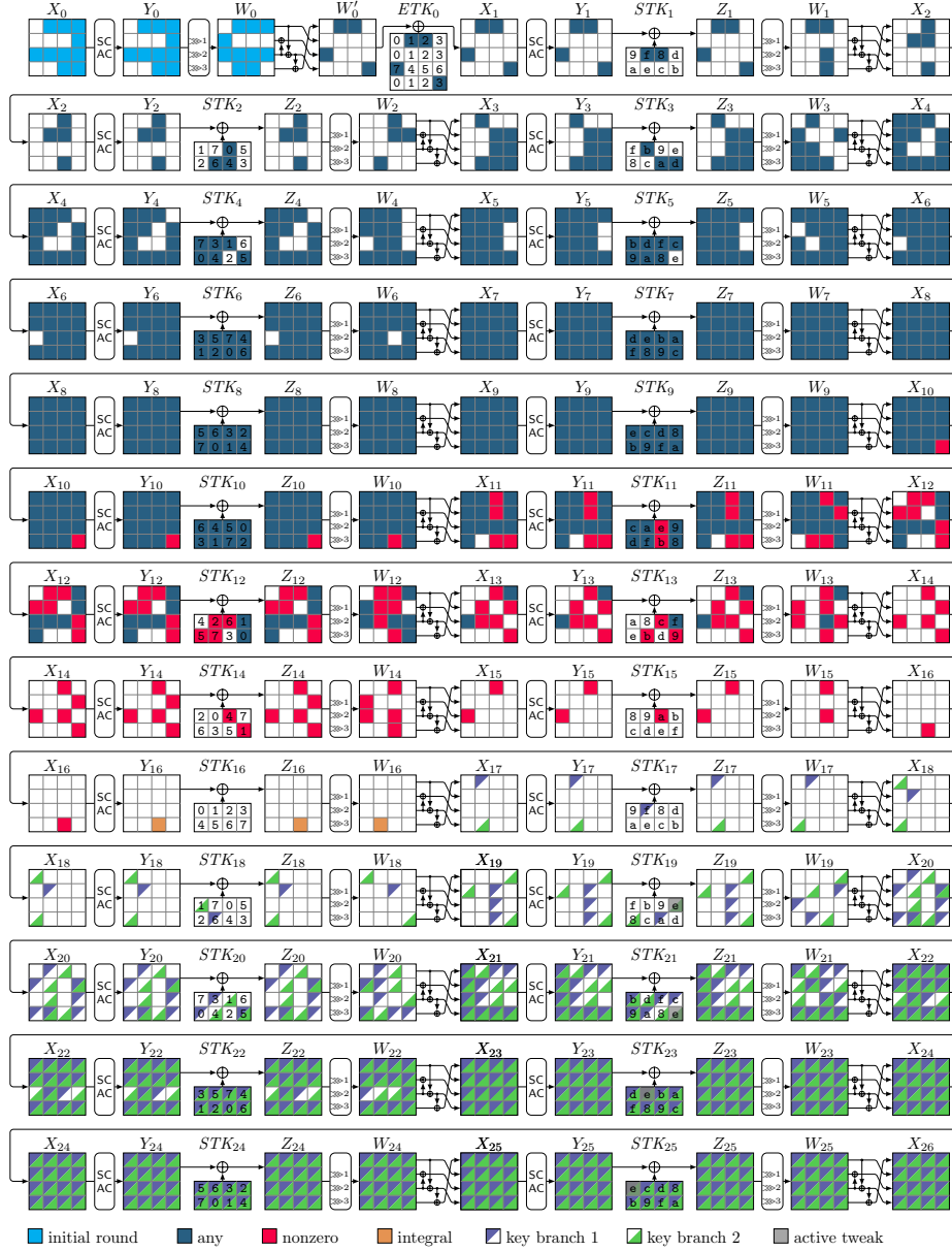
Fig. 15: ZC-based integral attack on 26 rounds of SKINNY- n-3n .
