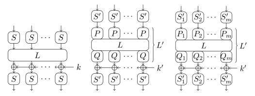
**Figure 1:** A keyed round function of an SPN with one additional S-box layer (left), an alternative representation of the round with  $S' = P^{-1} \circ S \circ Q^{-1}$  (middle), and an alternative representation of the round with  $S'_i = P_i^{-1} \circ S \circ Q_i^{-1}$  (right).
