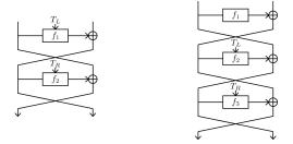
Fig. 1: The FEA-1 structure (left) and FEA-2 structure (right).
