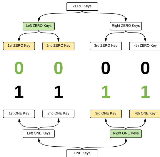
Fig. 8. Binary tree KDF-Lamport, where keys are derived via a Merkle tree structure.
