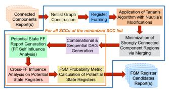
Fig. 6: *Netlist Graph Topological Analyzer* framework. It generates a list of FSM register candidates with the maximum values of *FPM*. Later stages use these register candidates to reconstruct the control FSM netlists.
