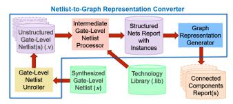
Fig. 5: *Netlist-to-Graph Representation Converter* framework. It generates the associated graph representations of the recognized unstructured gate-level netlists from the input gate-level netlist, which can be either hierarchical or flattened.
