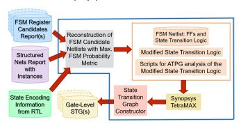
Fig. 8: Framework of the *Gate-Level State Transition Graph Extractor* module. It performs ATPG-based analysis to extract the gate-level STGs of the detected control FSMs.
