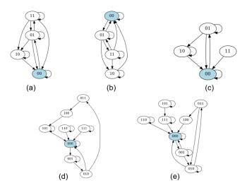
Fig. 12: The obtained 5 gate-level STGs of the control FSMs of *OpenRISC 1200* CPU [62]. All the control FSMs are encoded using the *Binary* state encoding. However, *FSMx* failed to extract the gate-level STGs since the associated state transition logic circuits contain a massive number of primary inputs.
