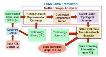
Fig. 4: Overview of the FSMx-Ultra framework. The framework analyzes the input synthesized gate-level netlist of a particular RTL design and yields the state transition graphs of the detected control FSMs.
