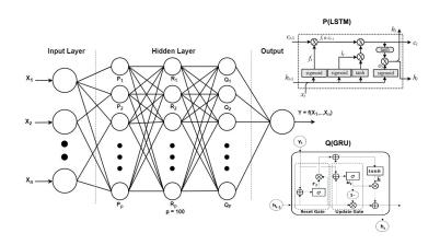
Fig. 4. LSTM-GRU Hybrid Model Architecture
