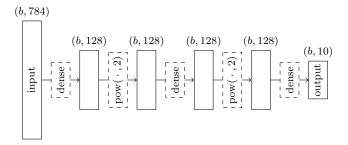
Fig. 23. Architecture of "network A" [1], [79]. The shape of the input and (intermediate) feature tensors is given above each tensor. *b* represents the batch size. Dashed boxes represent the network layers (dense layers, nonlinearities).
